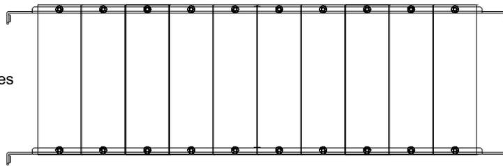
Optional 90° Brackets (to fix the frontpanel or rearpanel with the top and bottom cover)
