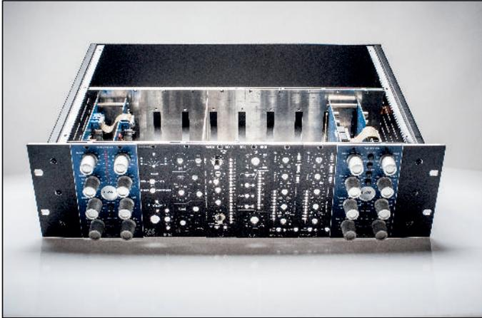
You can make an API500/51X rack out of an 3U enclosure, when using the mounting rails.
