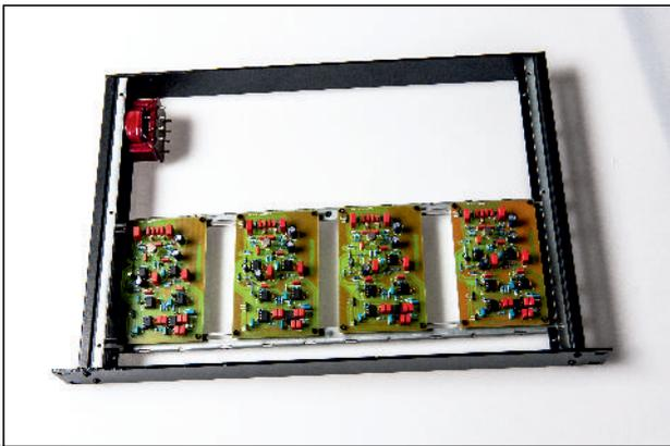
The mounting rail can be placed at the top and bottom position of the front and/or rearpanel. Countersink-holes in the side panel will hold the mounting rails in place. You can also move the mounting rails to any desired position.
